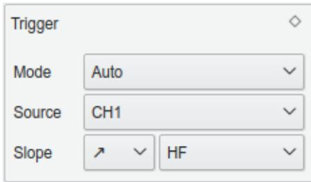
Triggering allows to display a stationary trace by fixing a rising or falling **Slope** of the signal of the selected **Source** channel to a defined position on the screen. The triggering is done in software by searching for the trigger condition in the sampled values and skipping the necessary amount of leading samples to position the trace accordingly.
