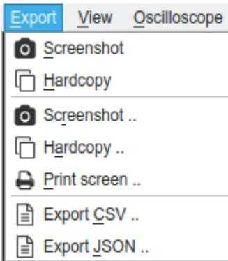
The Export CSV function allows to store the measured samples and the resulting spectral values as a \*.csv file (comma separated values).
