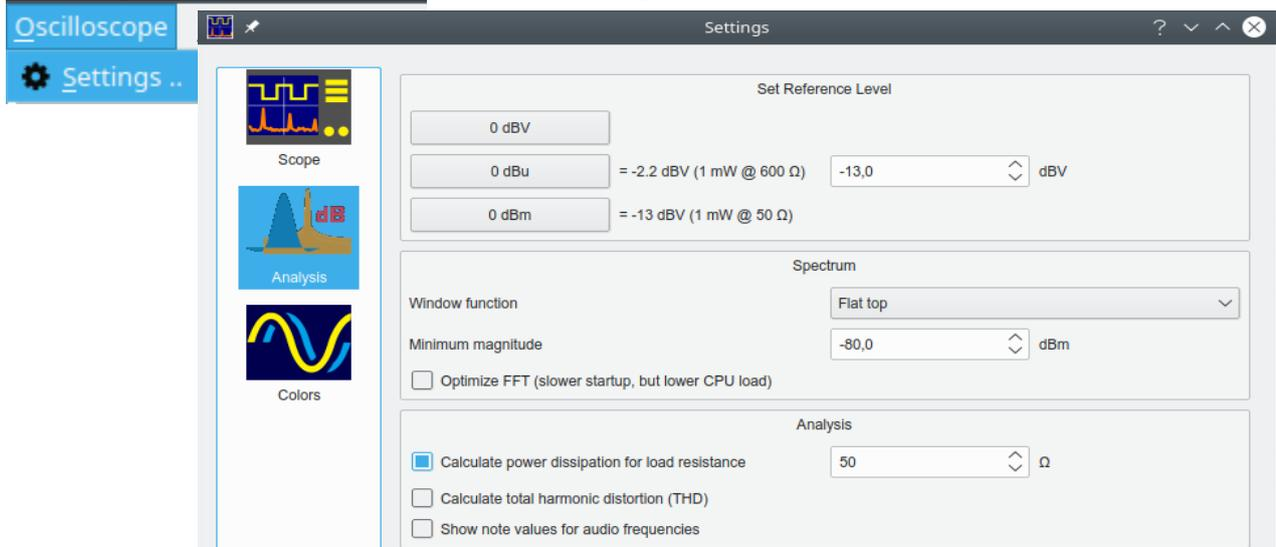
The default **Reference Level** can be set with the tree buttons on the left or by typing a value on the right. This doesn't change the input impedance, if you want to measure loaded signals, a capable dummy load must be connected to the scope input.
