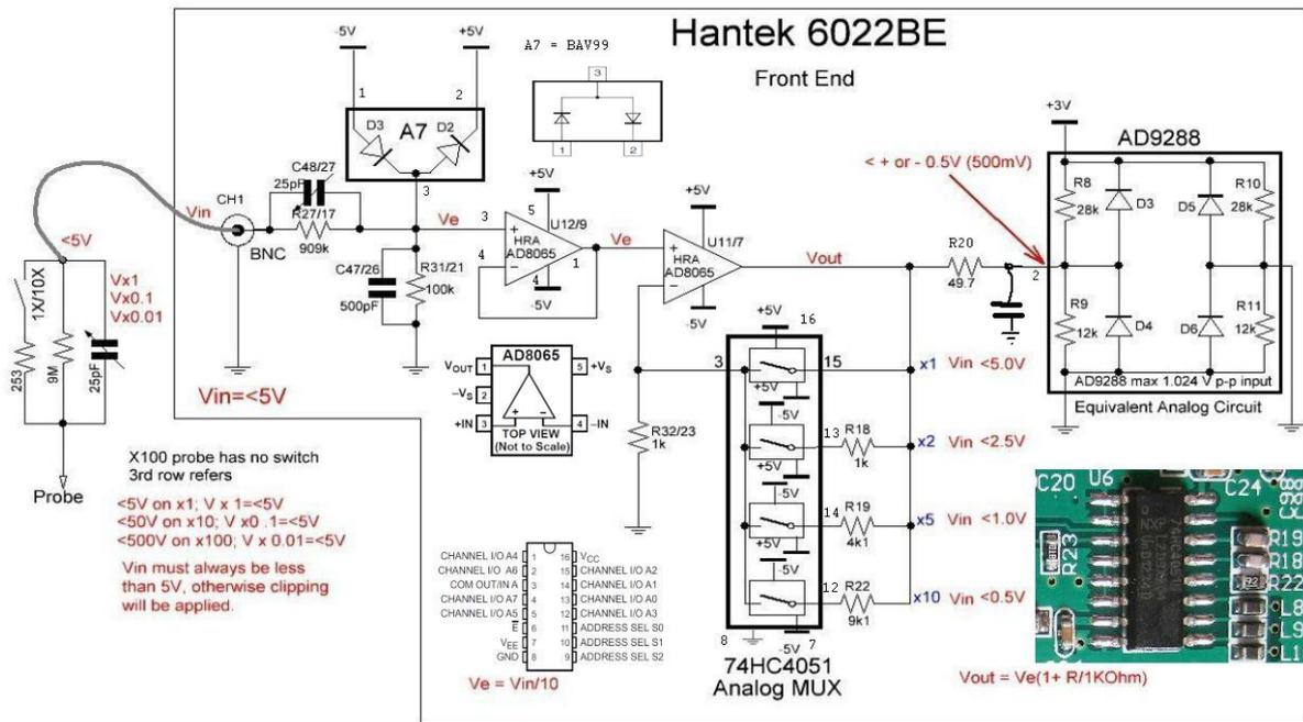
The input signal  $V_{in}$  is divided 1:10 by a frequency compensated resistors R27/17 and R31/21. Clamping diode A7 limits  $V_e$  to  $\pm 5$  V (equates  $V_{in} = \pm 50$  V). U11/7 together with the analog multiplexer amplifies  $V_e$  by 1X, 2X, 5X or 10X ( $V_{out}$ ).
