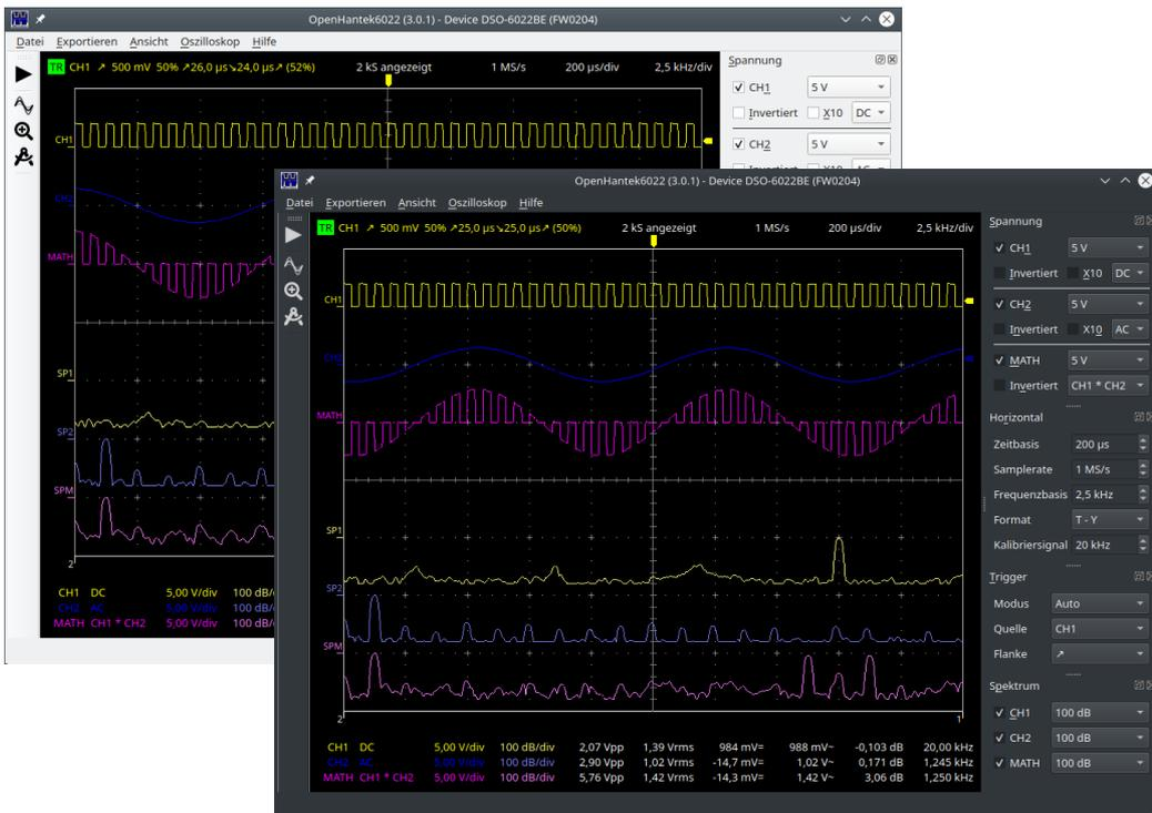
The colors of the traces on the screen as well as the exported png / pdf documents can be adjusted individually in the menu Oscilloscope / Settings / Colors.
