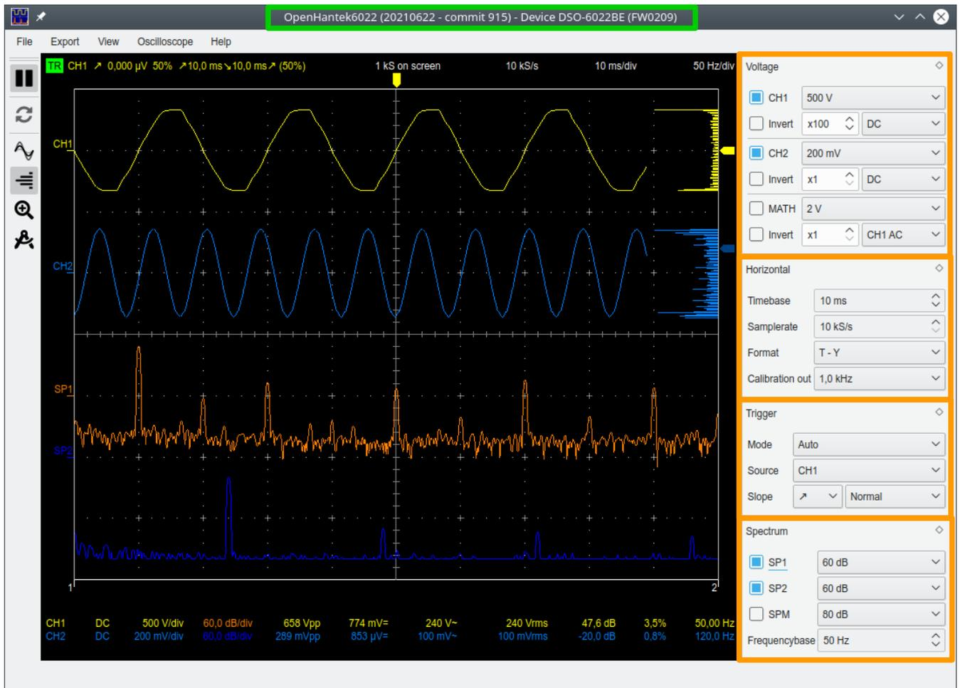
The scope functions can be controlled by the four docks (marked orange) on the right: Voltage, Horizontal, Trigger and Spectrum. These docks can be floated, rearranged or tabbed by grabbing their title lines, dragging and dropping. Drop on the screen to float it or move it over the docking area and drop it either on an empty blue space to rearrange it or drop it on another blue dock to tab both together. This way you can reduce the needed screen height when used on older computers or laptops.
