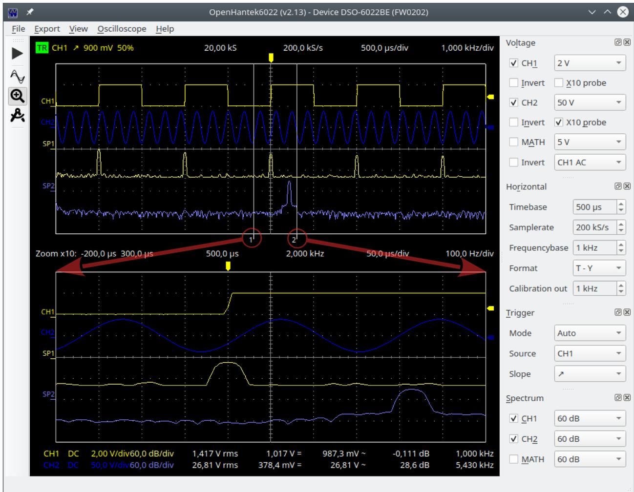
Mouse wheel scroll in the black border around the traces area changes the ratio of main to zoom window height between 1:1, 2:1, 4:1, 8:1 and 16:1.
