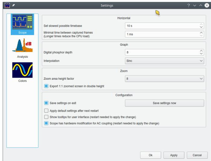
Longer hold-off time between captured frames allows to lower the CPU load, while faster sampling improves the triggering on rare events.
