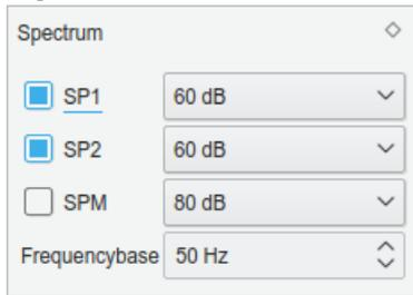
The program calculates the voltage spectrum of the three channels using the discrete FFT and displays the results if enabled.
